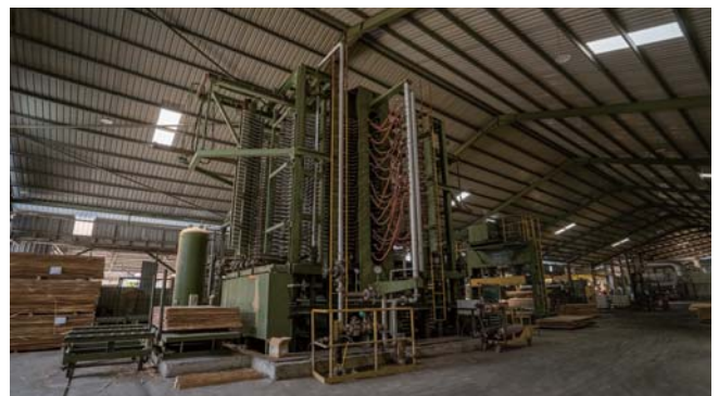
Hot pressing in Tan Chee Seng Sawmill Perak, Malaysia. Photo: Khairul nizam
